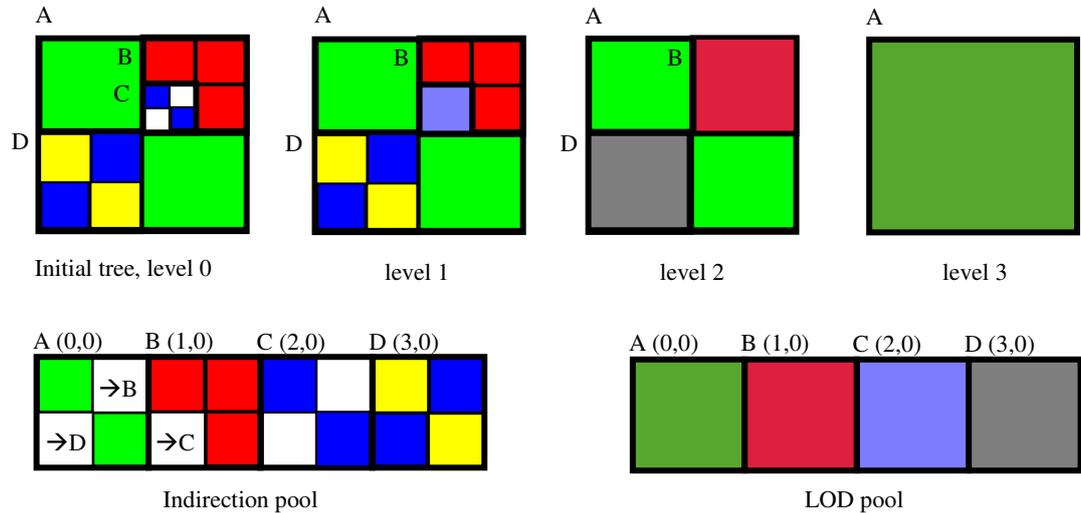
Figure 9: Example of tree with MIP-mapping
