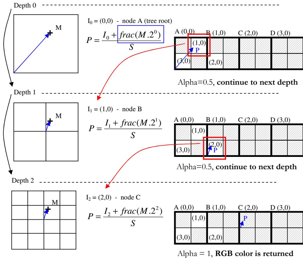
Figure 5: Example of tree lookup. At each step the value stored within the current node's indirection grid is retrieved. If this value encodes an index, the lookup continues to the next depth. Otherwise, the value is returned.
