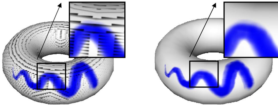
Figure 7: Artifacts introduced by straightforward linear interpolation (left). Corrected linear interpolation (right).
