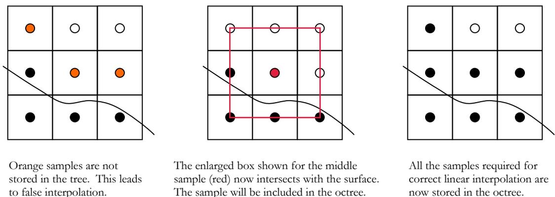
Figure 8: Modifying the tree creation to remove linear interpolation artifacts
