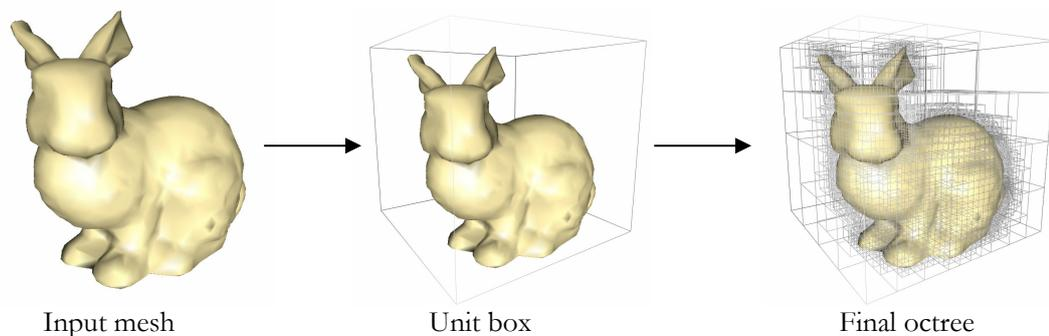
Figure 6: Building an octree around the mesh surface.
