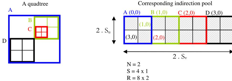
Figure 4: Storage in texture memory (2D case). The indirection pool encodes the tree. Indirection grids are drawn with different colors. The grey cells contain data.
